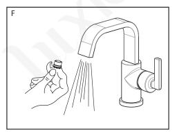
F. Remove the aerator with a small coin or a flat head screwdriver and let the water run for about 1 minute to clear any debris in the plumbing system. Check for leaks at all connections. Reinstall the aerator to complete the installation.
