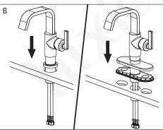
B. Use the flange for a single hole installation OR use the included deck plate to covert a 4 inch centerset hole pattern to a single hole pattern.
