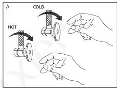
A. Shut off water supply at the valves. Remove the old faucet and clean the mounting surface for installation of the new faucet.
